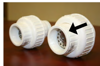
Figure 5 - In-line Union-Strainers. Install in the drain line upstream of the Air-Trap. This will aid in preventing debris from entering trap. The arrow shows the direction of water flow, into the strainer basket.
