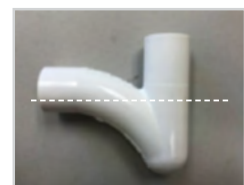
Figure 3b: Molded 3/4" P-Trap
