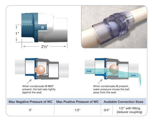
Note: The attached drawings represent traps that operate under negative pressure. Never connect condensate drain directly to a sanitary drain line.
