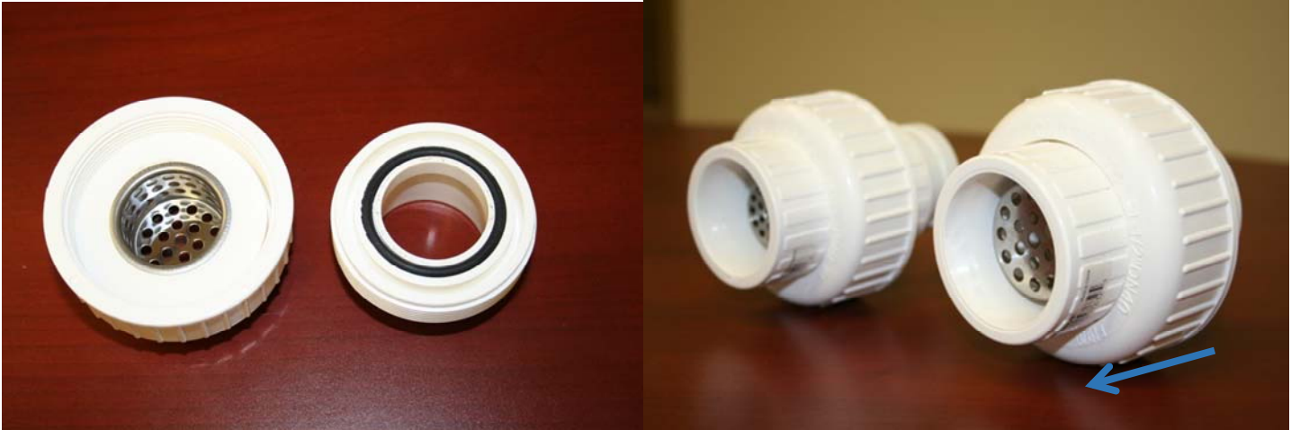
Figure 8 In-line Union-Strainers. Install in the drain line upstream of the Air-Trap. This will aid in preventing debris from entering trap.
