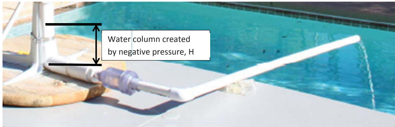
Figure 4 Des Champs N-Series Air-Trap undergoing tests at the Des Champs Technologies Las Vegas, NV test facility. Testing videos showing the operation of the trap are viewable at www.deschampstechnologies.com , then go to N-Series and then to N-Series YouTube Presentation
