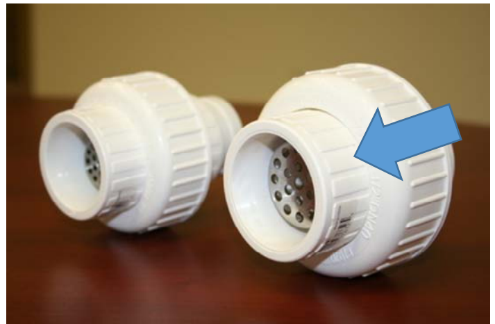
Figure 5: In-line Union-Strainers. Install in the drain line upstream of the Air-Trap. This will aid in preventing debris from entering trap. The arrow shows the direction of water flow, into the strainer basket.
