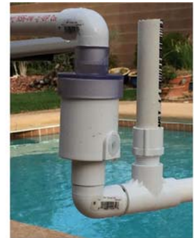
Figure 6 N-SERIES Air-Trap when installed vertically can operate properly up to 3" of positive pressure.
