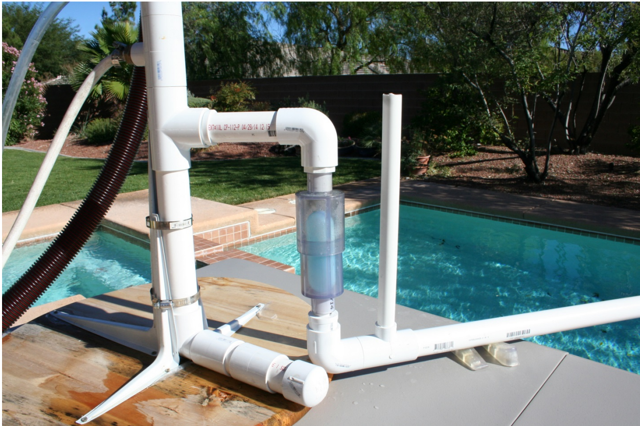
Figure 6. Positive Pressure P-Series HVAC Air-Trap undergoing tests at the Des Champs Technologies Las Vegas, NV test facility. Testing videos showing the operation of the trap are viewable at www.deschampstechnologies.com , then go to P-Series and click on the link P-Series YouTube Presentation
