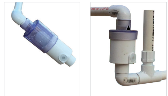
Figure 5 - P-Series Air-Trap installed at 45° angle can reduce trap height by 30% and operate at up to 5" of positive pressure.
