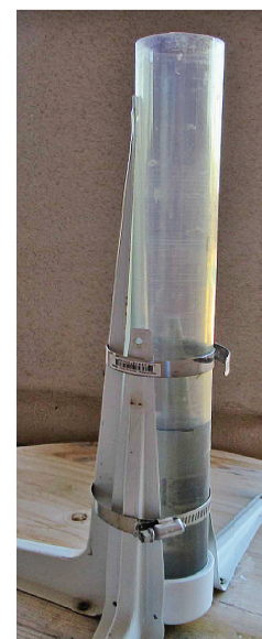
Figure 6: Test stand for measuring evaporation of water at different conditions
