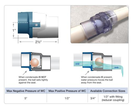
Note: The attached drawings represent traps that operate under negative pressure. Never connect condensate drain directly to a sanitary drain line.
