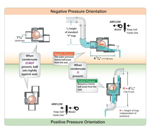
Note: The attached drawings represent traps that operate under negative or positive pressure. Never connect condensate drain directly to a sanitary drain line.
