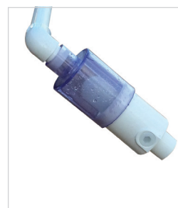
Figure 5 - P-Series Air-Trap installed at 45° angle can reduce trap height by 30% and operate at up to 5" of positive pressure.
