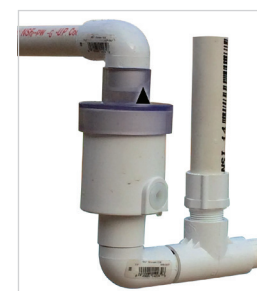
Figure 6 - N-Series Air-Trap when installed vertically can operate properly up to 3" of positive pressure.
